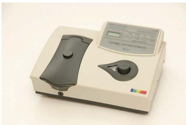
Using a reconfigured grating monochromator from the successful M105 and M106 models, the M107 offers more performance and versatility with only a modest price difference. The large sample compartment allows the use of a wide range of accessories, including a 4-position cell changer with holder for cell pathlengths up to 50mm. A membrane keyboard positioned next to the large, clear LCD display allows the operator to rapidly switch between %T, Abs and Concentration modes and to set Zero Abs.
